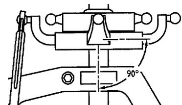
Don't use the pitch gauge until you have installed all the servo horns and pushrods. Pitch settings usually are the last step in completing the basic setup for the helicopter just prior to making the first test flights.
