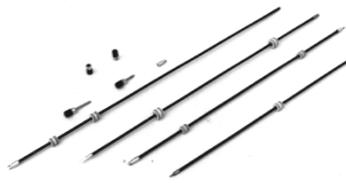
Replace the wire drive system improving tail rotor response, especially if using a heading hold gyro.
